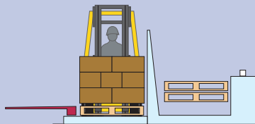
1. The pallet load is placed in the station and the forks withdrawn from the pallet.
